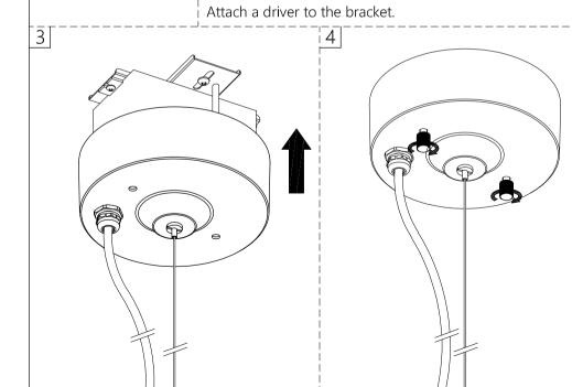
Fix it with fixing parts.
