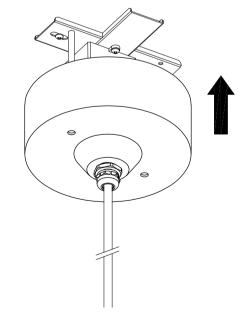
Attach the flange to the bracket.
