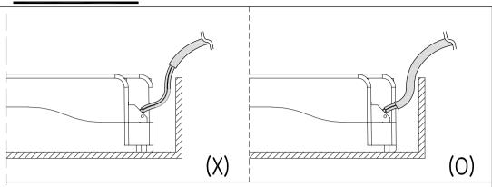
\* The cable protective jacket have to be removed only near terminal block to ensure uncovering basic insulation wire not touch the metal around.
