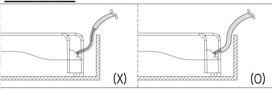
\* The cable protective jacket have to be removed only near terminal block to ensure uncovering basic insulation wire not touch the metal around.
