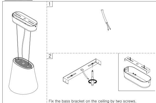
\* The cable protective jacket have to be removed only near terminal block to ensure uncovering basic insulation wire not touch the metal around.
